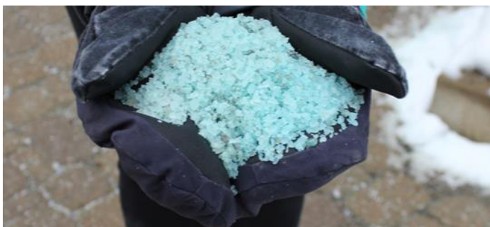
Figure 1. Rock salt treated with a magnesium chloride coating
